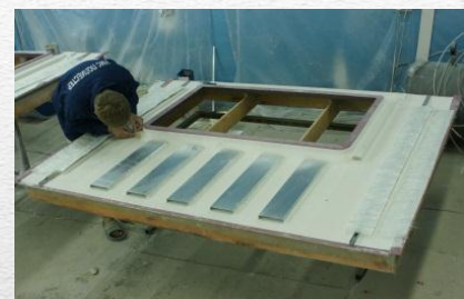
Process 5. Pad gluing
