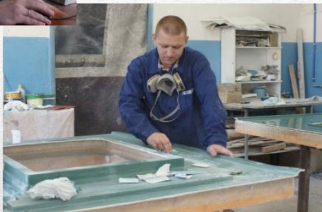
Process 2. Putting priming coat and gel coat onto the ready tool
